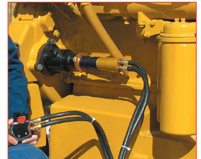
A B006PVR374-03-31P barring motor using pendant control, slow turning a Caterpillar 3408 engine.
